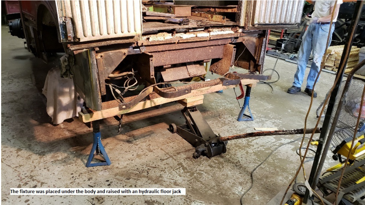
The fixture was placed under the body and raised with an hydraulic floor jack
