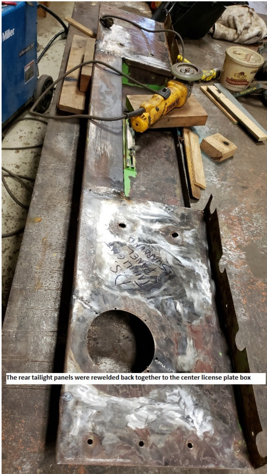
The rear tail light panels were rewelded back together to the center license plate box
