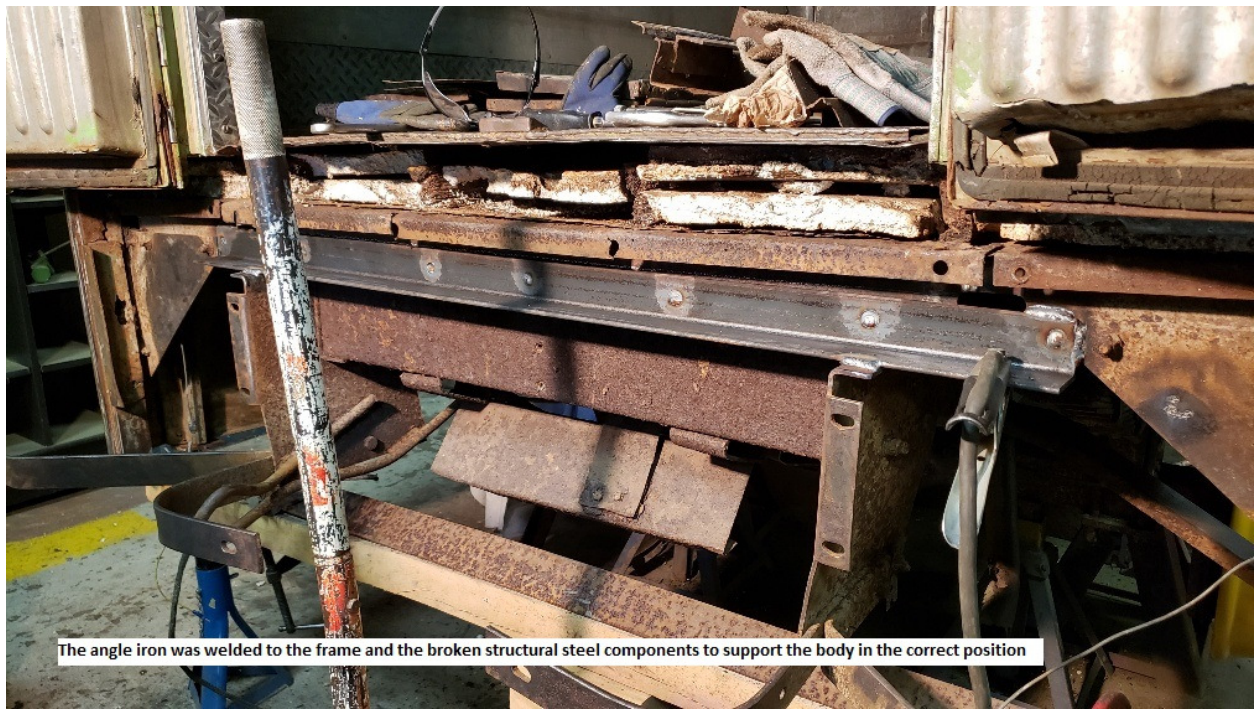
The angle iron was welded to the frame and the broken structural steel components to support the body in the correct position
